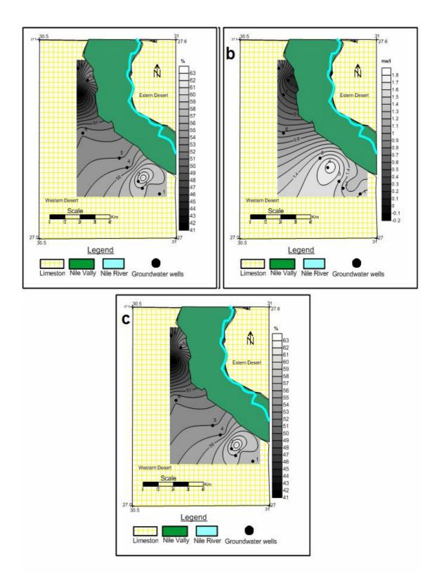
**Fig. (6):** The contour map of RSC(meq/l) (a), RSCB(meq/l) (b) and SSP(c) (%) in the study area.
