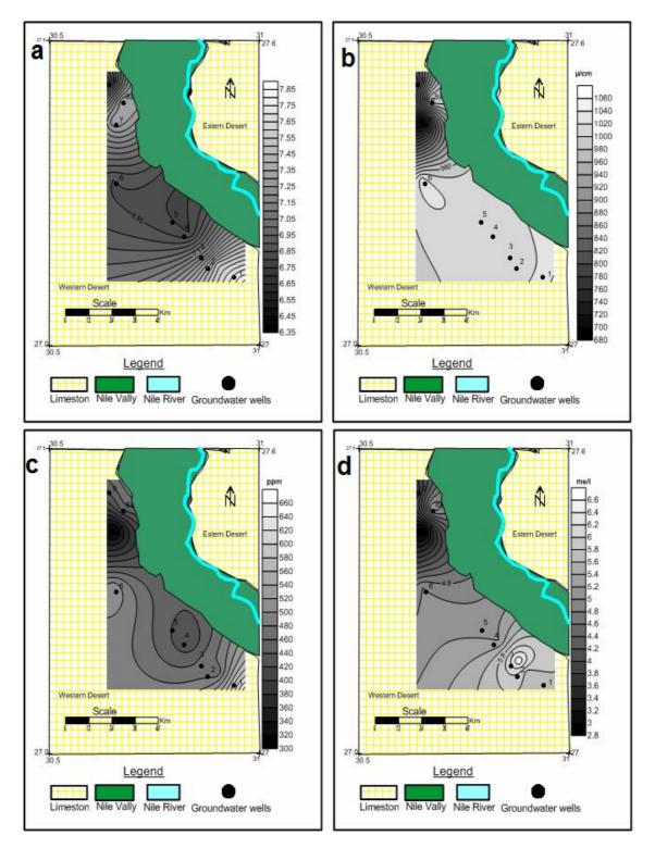
Fig. (5): The contour map of pH `(a) , EC ( $\mu$ S/cm) (b), TDS (mg/l) (c) , and SAR(d) in the study area.
