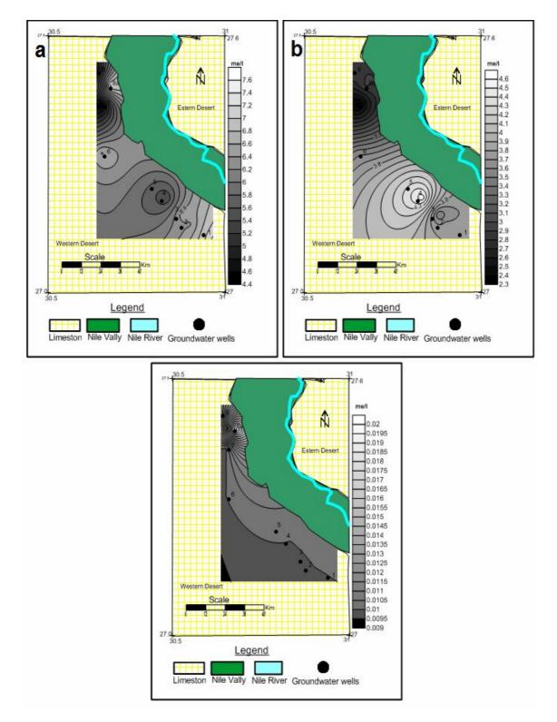
Fig. (4): The contour map of Cl(a),  $HCO_3(b)$ , and  $SO_4(c)$  meq/l in the study area.
