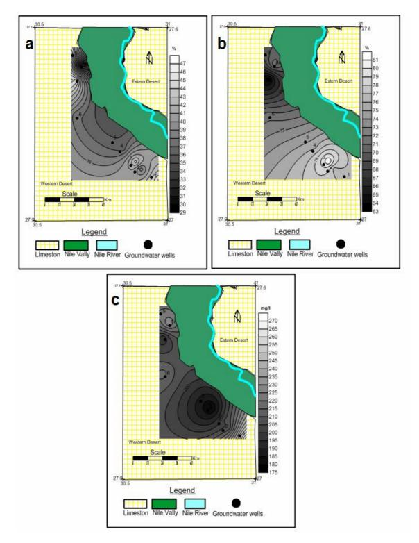
Fig. (7): The contour map of MH (%)(a), PI (%)(b) and TH (mg/l)(c) in the study area.
